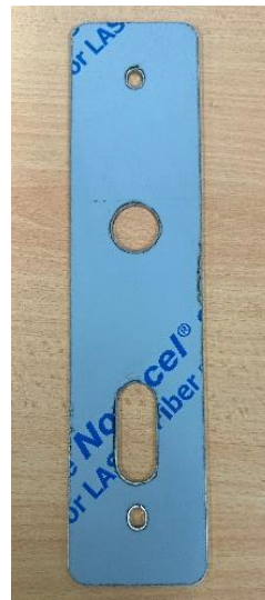
Figure 3 Latch edge side view of the tested hardware Figure 4 Scar plate preinstallation
